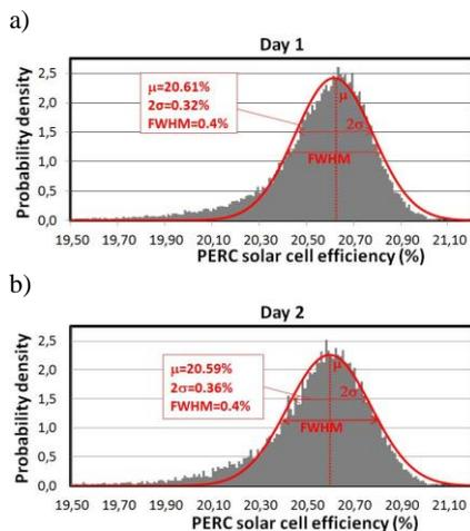
**Figure 7:** Probability density of PERC solar cell efficiency for day 1 (a) and day 2 (b), where for both days based on the normal distribution the average solar cell efficiency is at 20.6% and FWHM is determined to be on 0.4%. FWHM is the width of the distribution where the distribution is equal to half of the maximum.
