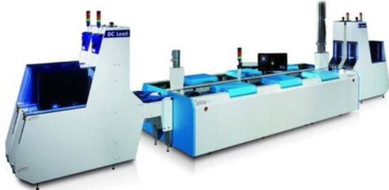
**Figure 2:** InPassion ALD equipment of SoLayTec, which consists of six modules, with loader and unloader.
