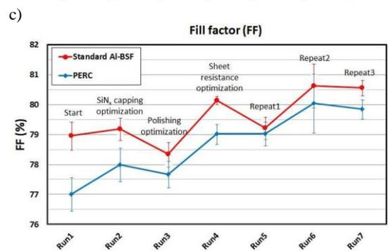
**Figure 5:** Open circuit voltage ( $V_{\text{oc}}$ ) (a), short circuit current density ( $j_{\text{sc}}$ ) (b), and fill factor (FF) (c) for PERC solar cell and standard Al-BSF solar cell for the different optimization runs and repeat runs.
