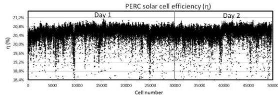
**Figure 6:** Absolute solar cell efficiency of the first 2 days of the production ramp-up of PERC. A stable efficiency of  $(20.5 \pm 0.3)\%$  has been achieved.
