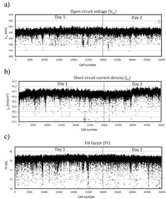
**Figure 8:** Open circuit voltage ( $V_{oc}$ ) (a), short circuit current density ( $j_{sc}$ ) (b), and fill factor (FF) (c) of the first 2 days of the production ramp-up of PERC.
