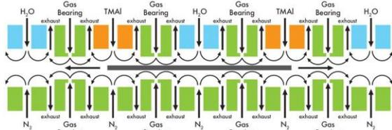
**Figure 3:** Schematic cross section of the injector head of the spatial ALD reactor.
