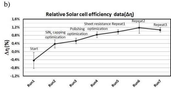
**Figure 4:** Absolute solar cell efficiency (a) and the solar cell efficiency of PERC and Al-BSF solar cell relative to each other (b).
