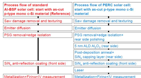
**Figure 1:** Processing flows for the Al-BSF solar cell and PERC solar cell.
